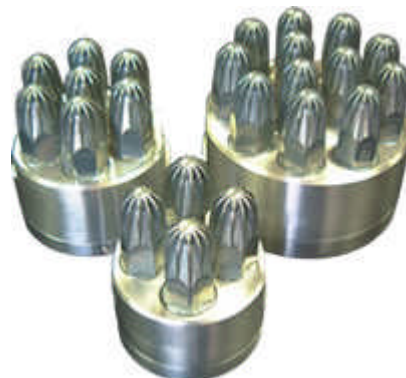
Super Air Nozzle Cluster 3.2 - 9.8 Pfund Kraft (1451 - 4445 g) 56 - 168 SCFM (1585 - 4754 l/min) Zink/Aluminium
