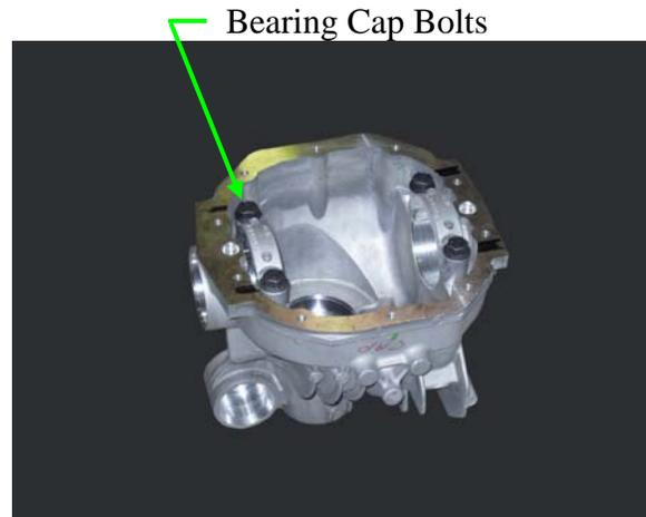
Two large bearings are part of drive train differential assemblies. The manufacturing process involves drilling and tapping holes and the assembly of the retaining bolts that hold the bearings in place. The bolt holes are blind so they tend to collect chips and other foreign material during machining.
