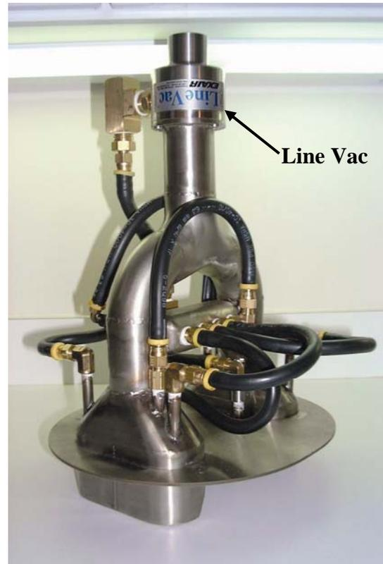
A blow-off/vacuum system incorporating **four EXAIR Model 1001 blow off nozzles** and an **EXAIR Model 6083 Line Vac** is automatically lowered to the differential housing just after machining but before assembly. The fixture cleans out the holes and safely vacuums the chips and debris away for deposit in a remotely positioned **EXAIR Model 6193 Chip Vac** (not shown).
