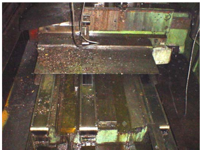
Chips seen on slide ways
