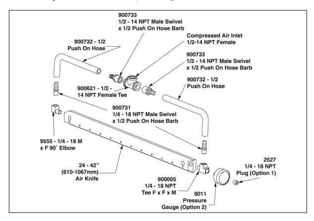
Pipe thread sealant should be applied to all threads (small packet included). Avoid the inside diameter of the fitting so it does not enter into the Air Knife.
