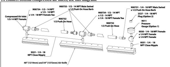
Pipe thread sealant should be applied to all threads (small packet included). Avoid the inside diameter of the fitting so it does not enter into the Air Knife.
