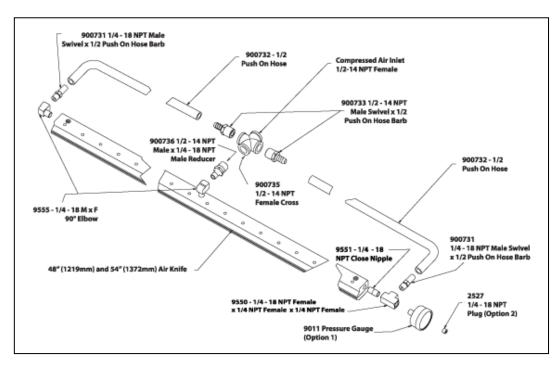
Pipe thread sealant should be applied to all threads (small packet included). Avoid the inside diameter of the fitting so it does not enter into the Air Knife.
