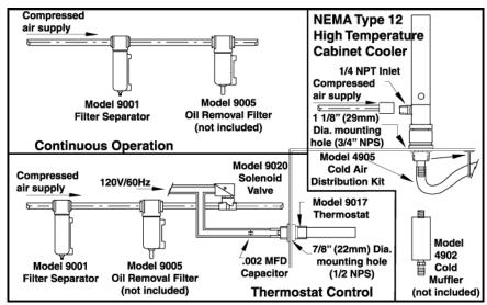
High Temperature Cabinet Coolers are rated for a maximum temperature of 200°F (93°C)
