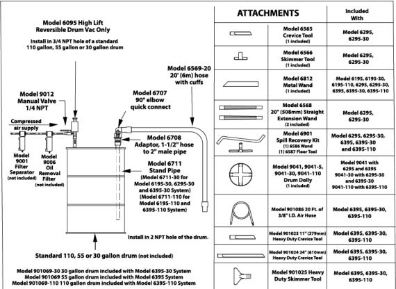
Note: The High Lift Reversible Drum Vac System must be used with a closed head steel drum with a minimum wall thickness of 1.3mm (18 gauge) and in good condition.
