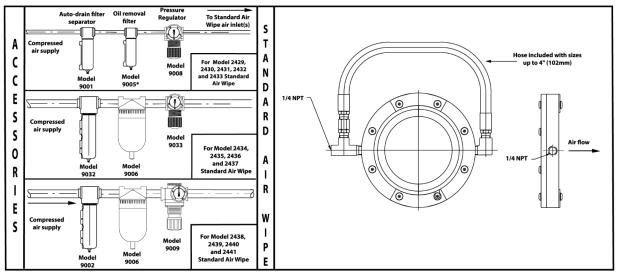
\* Use Model 9006 Oil Removal Filter for Standard Air Wipes that are 3" (76mm) and larger
