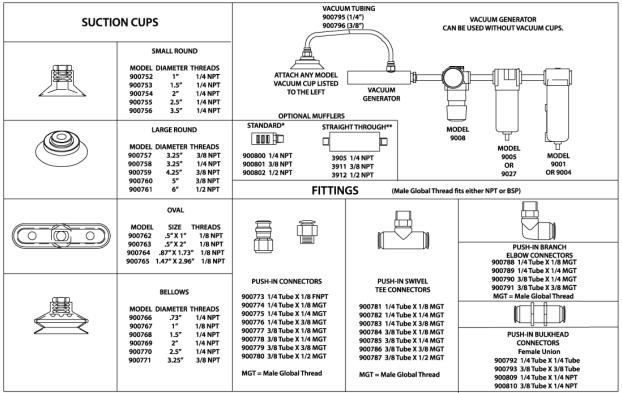
\*Max Pressure 150 psig (10 bar) Operating Temp 35°F-120°F (2°C-49°C)
