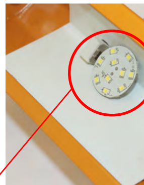
Led lamp 12VAC-10/30VDC
