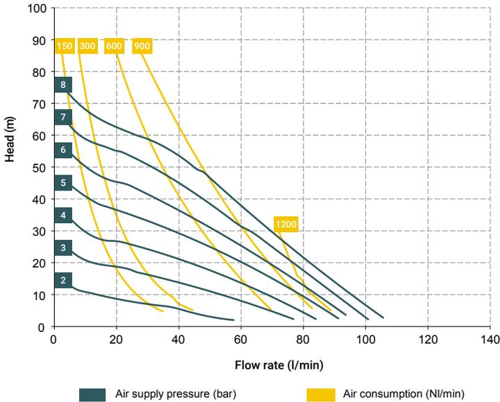
\* The curves and performances refer to pumps with immersed suction and open delivery outlet with water at 20 °C and vary according to the composition materials.
