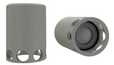
Foot valves are designed to be installed vertically at the end of the suction pipes of centrifugal and pneumatic pumps. They function as check valves that prevent the suction hose from emptying so that the pumps remain always primed.
