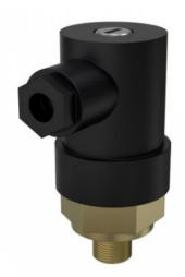
This is a device that is installed on the pneumatic circuit of diaphragm pumps. It measures the number of strokes performed by the diaphragms and therefore the number of cycles. Pump cycle counter can be used to activate various types of controls, such as for example, the litres of liquid delivered by the pump, according to its displacement capacity, and to remotely control its operation.
