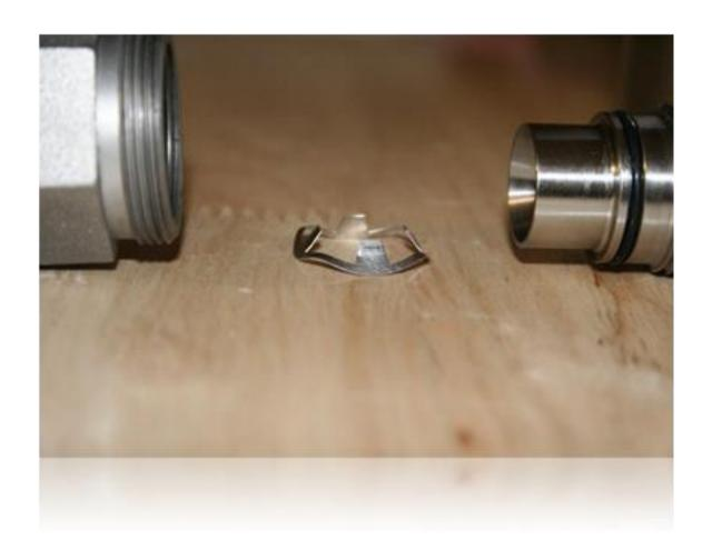
► Carefully remove the spacer from the pump body and clean it with a mild cleaning or degreasing agent.
