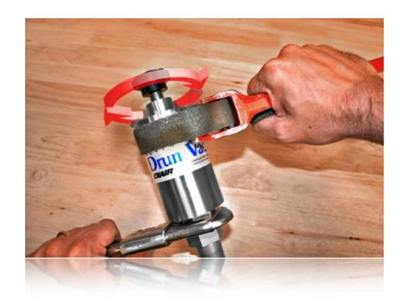
To remove the muffler, hold the hex body with a wrench while unscrewing the cylindrical muffler to the left using a strap wrench.
