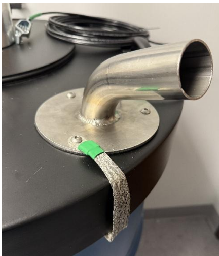
Figure 3: Top View of Ground Strap Installation
